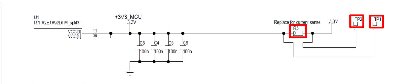
Figure 60. MCU Current Measuring Points (Circuit Diagram)
