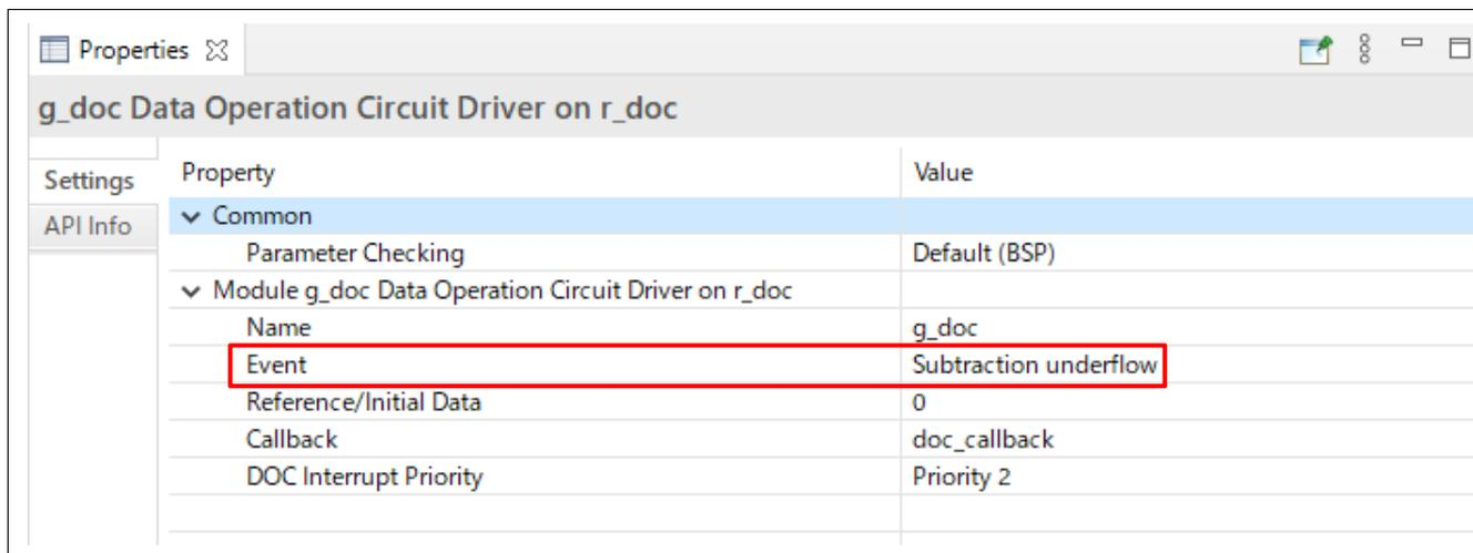
**Figure 20. DOC Function Settings on FSP Configurator**
