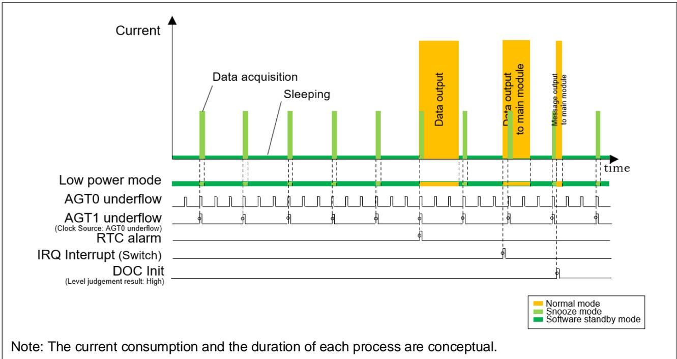
**Figure 2. RA2E1 Conceptual Diagram of Operation Mode and Current Consumption**
