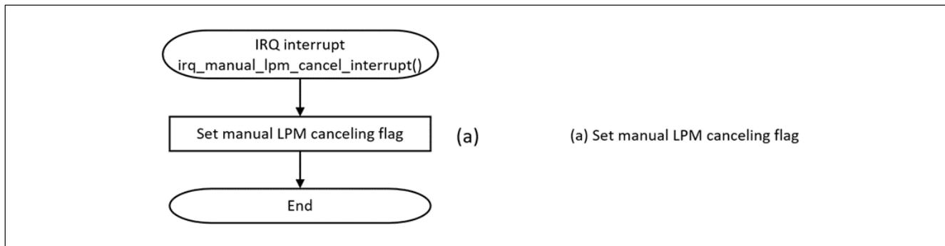
**Figure 49. IRQ Interrupt Processing**
