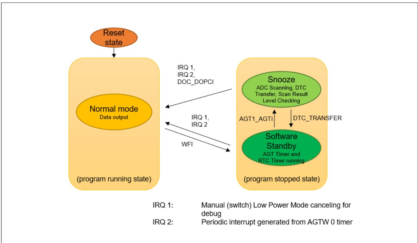
**Figure 3. RA2E2 MCU Status and Mode Transition Events**
