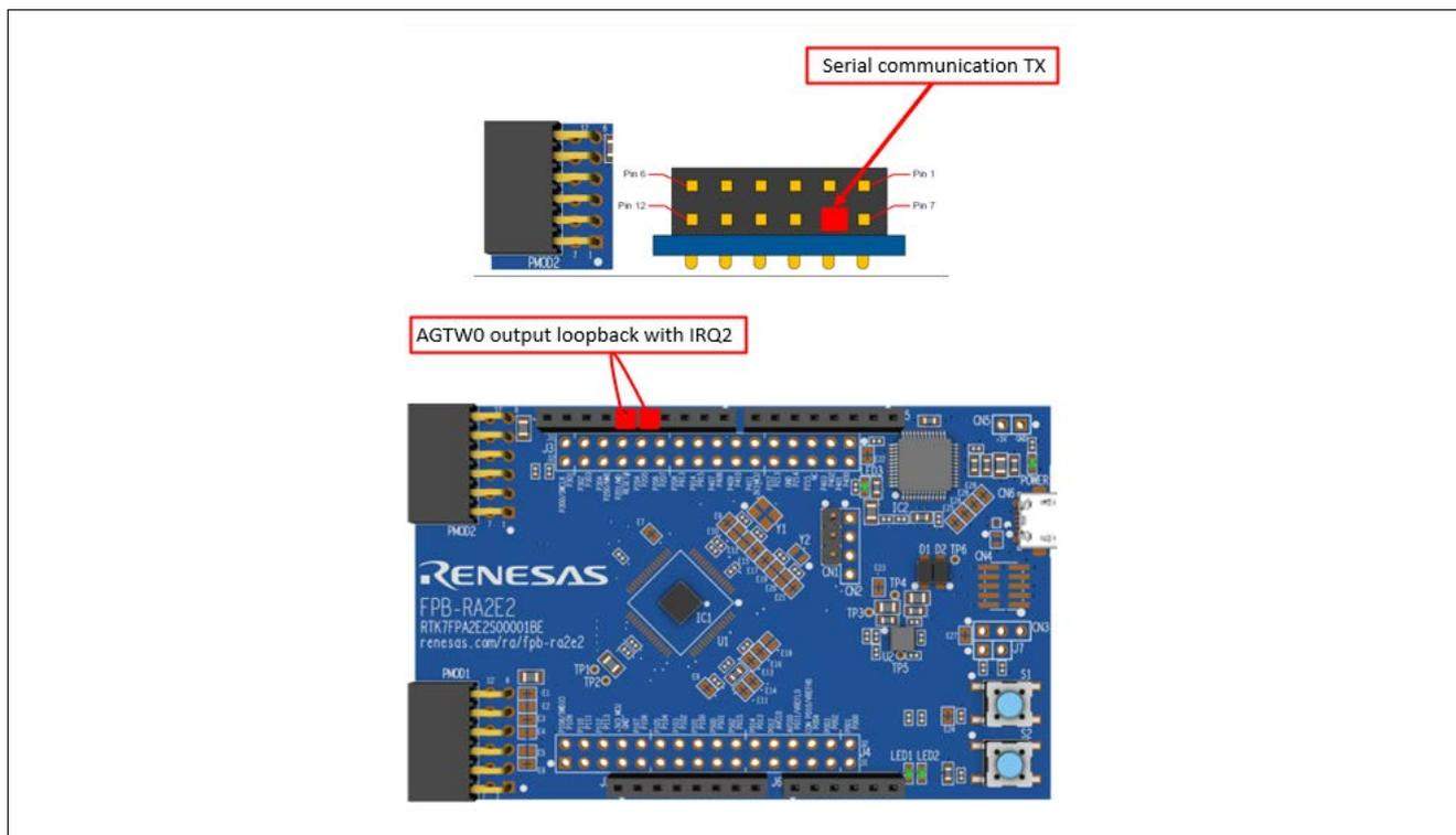
Figure 37. FPB-RA2E2 Connecting to the External Equipment
