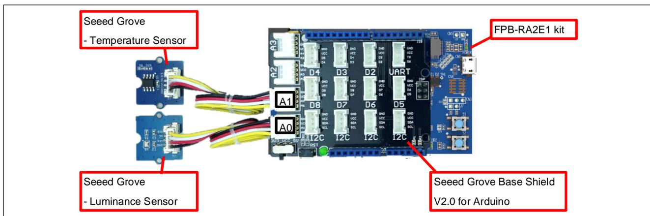
Figure 34. FPB-RA2E1 Sensor Connection
