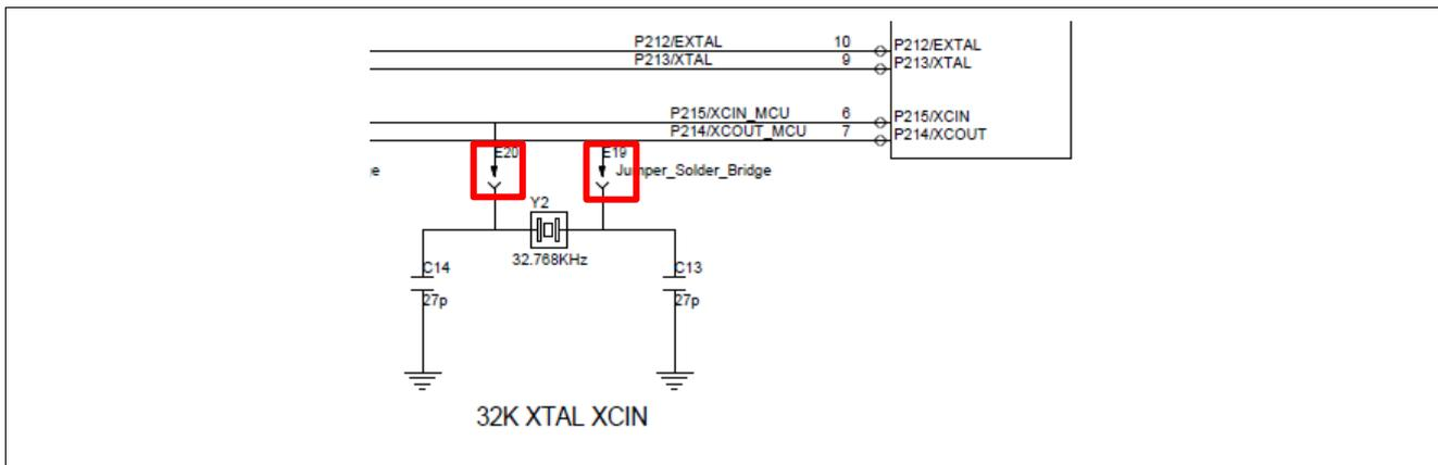
Figure 40. Solder Jumper for External Oscillator Connection (Circuit Diagram)
