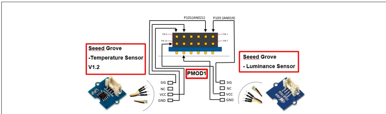
Figure 12. FPB-RA2E2 kit PMOD1 Connection with Analog Sensors
