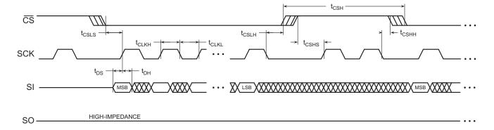
Figure 40. Serial Input Timing
