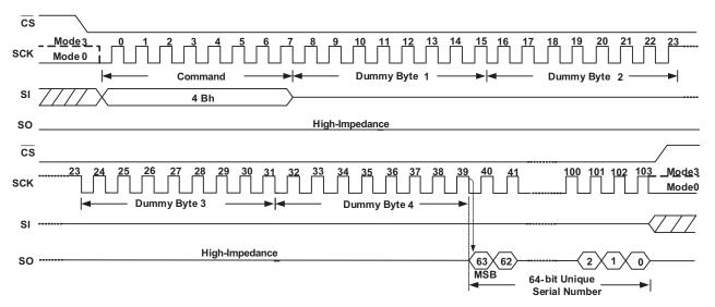
Figure 24. Read Unique ID Timing (SPI Mode)
