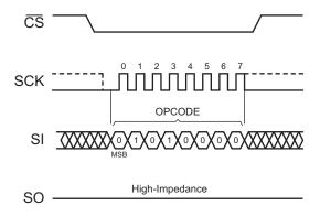
Figure 31. Write Enable for Volatile Status Register
