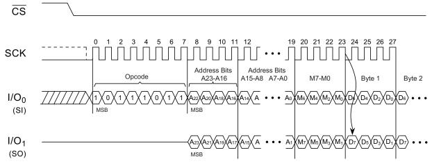
Figure 9. Dual I/O Read Array (Initial command or previous M5,M4 ≠ 1,0)
