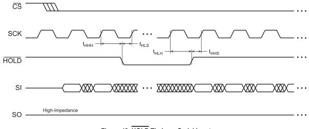
Figure 43. HOLD Timing – Serial Input
