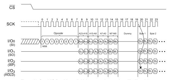
Figure 12. Quad-I/O Read Array (Initial command or previous M5, M4  $\neq$  1,0)
