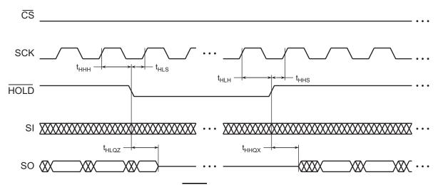
Figure 44. HOLD Timing - Serial Output
