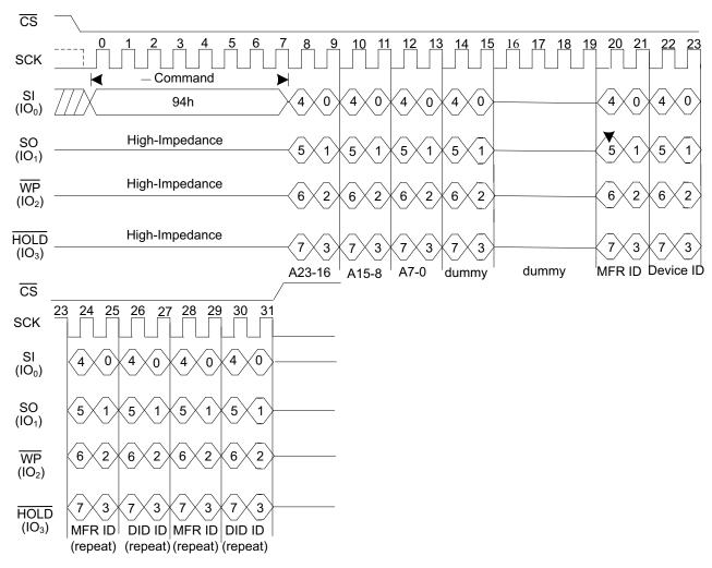
Figure 35. Quad I/O Read Manufacture ID / Device ID Timing
