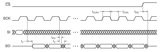
Figure 41. Serial Output Timing
