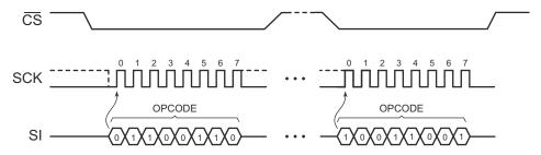
Figure 23. Enable Reset (66h) and Reset Device (99h) Command Timing (SPI Mode)
