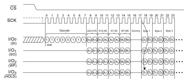
Figure 15. Quad I/O Word Fast Read Timing (Initial Command Set M5, M4 ≠ 1,0) SPI Mode
