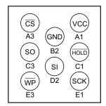
Figure 2. 8-ball WLCSP (3 x 2 x 3) — Bottom View
