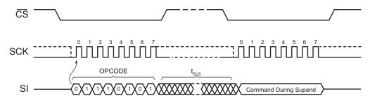
Figure 22. Erase/Program Suspend Timing
