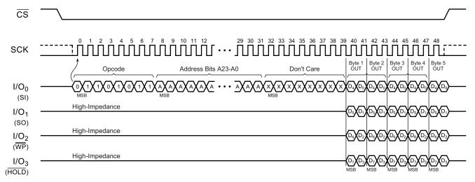
Figure 11. Quad-Output Read Array
