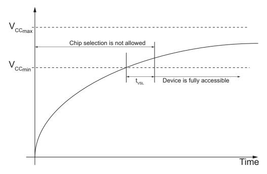
Figure 39. Power-Up Timing and Voltage
