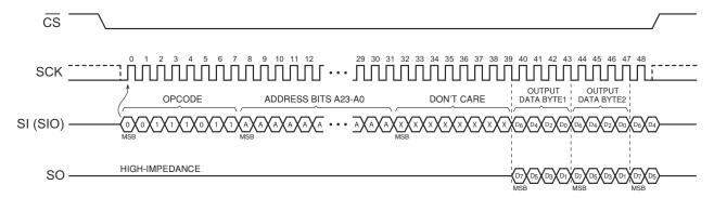
Figure 8. Dual-Output Read Array
