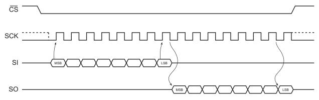
Figure 5. SPI Mode 0 and 3
