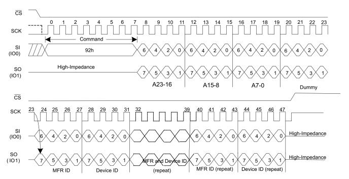
Figure 34. Dual I/O Read Manufacture ID/ Device ID Timing
