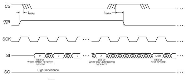
Figure 42. WP Timing for Write Status Register Command When BPL = 1
