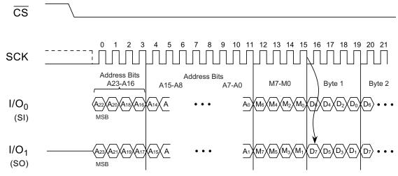
Figure 10. Dual-I/O Read Array (Previous command set M5, M4 = 1,0)
