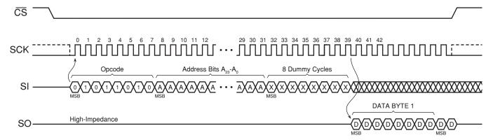
Figure 17. Read Serial Flash Discoverable Parameter Command Timing
