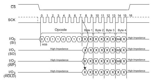
Figure 14. Set Burst with Wrap Timing (SPI Mode)
