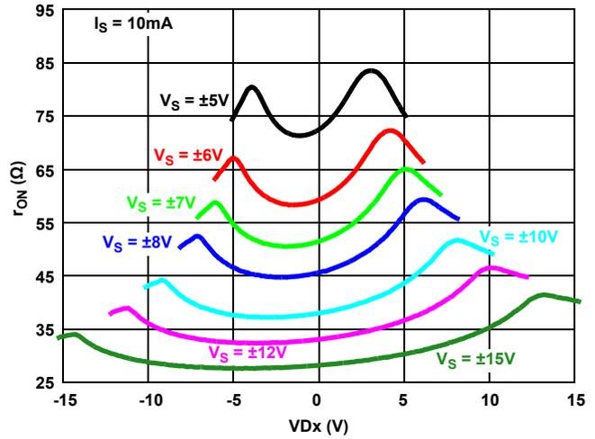
Figure 12.  $r_{ON}$  vs Signal Level vs Supply Voltages
