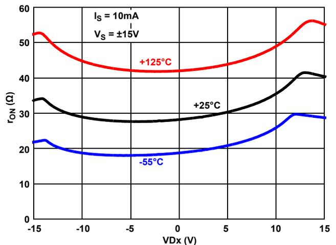
Figure 2.  $r_{ON}$  vs Signal Level vs Temperature
