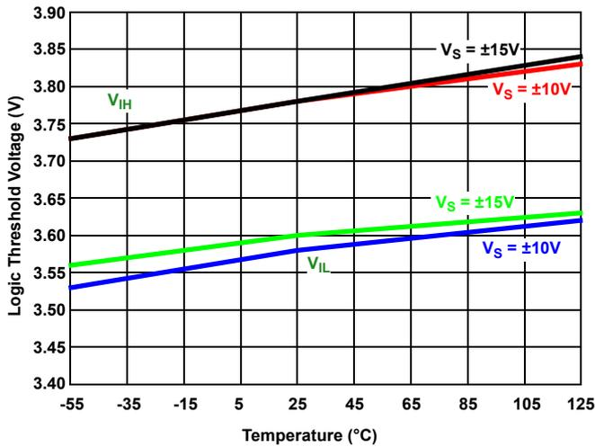
Figure 19.  $V_{IH} / V_{IL}$  vs Temperature vs Supply Voltages
