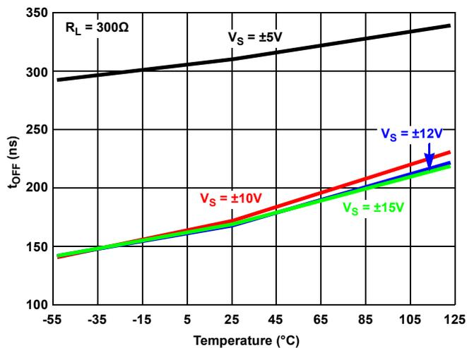
Figure 15.  $t_{OFF}$  vs Temperature vs Supply Voltages
