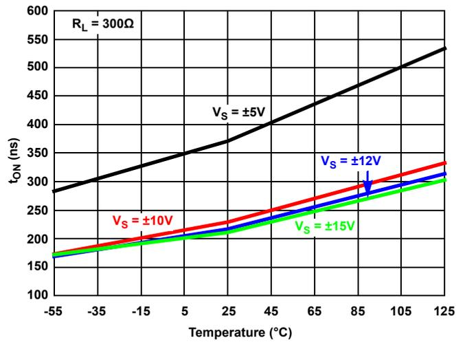
Figure 14.  $t_{ON}$  vs Temperature vs Supply Voltages
