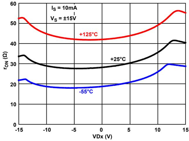
Figure 11.  $r_{ON}$  vs Signal Level vs Temperature
