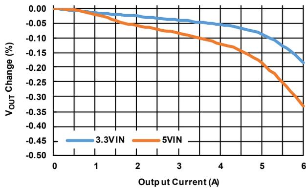
Figure 20.  $V_{IN}$  Load Regulation 1.2V  $V_{OUT}$
