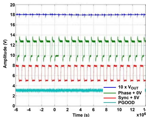
Figure 37. Set Response with 3V Input,  $\Delta V_{OUT} < 1\%$
