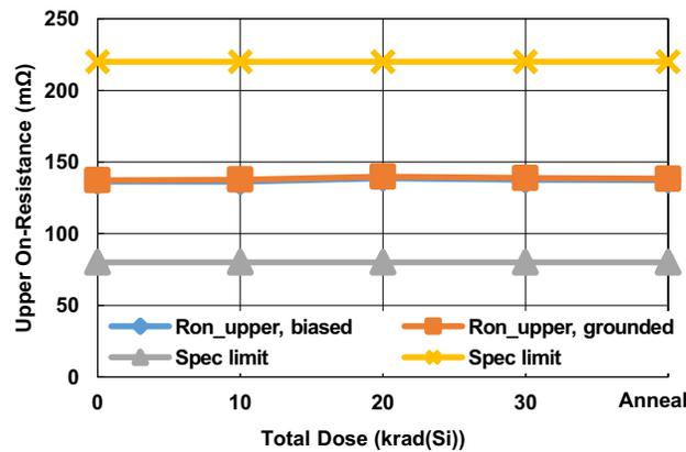
Figure 35. Upper  $r_{DS(ON)}$  vs TID
