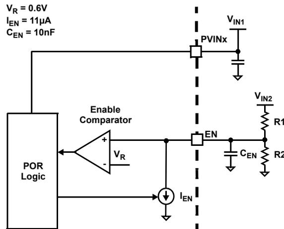
Figure 26. Enable Circuit
