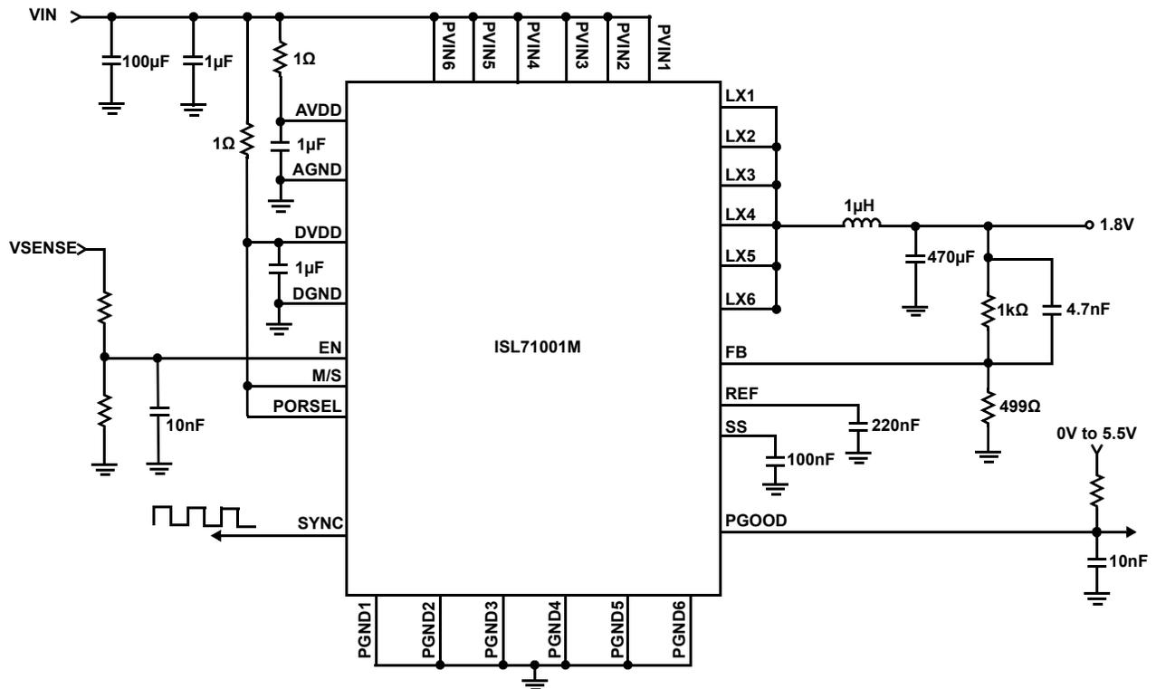
Figure 38. Simplified Schematic of ISL71001M SEE Test Circuit
