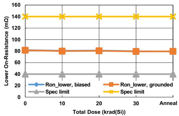
Figure 34. Lower  $r_{DS(ON)}$  vs TID
