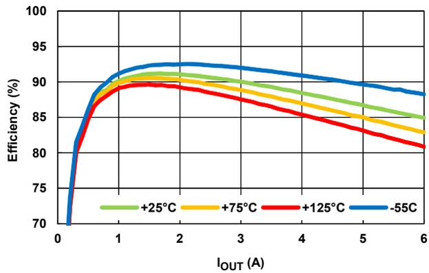
Figure 9. 3.3V  $V_{IN}$  Efficiency, 1.2V  $V_{OUT}$  Over Temperature
