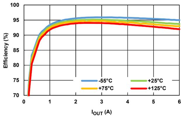
Figure 8. 5V  $V_{IN}$  Efficiency, 3.3V  $V_{OUT}$  Over Temperature
