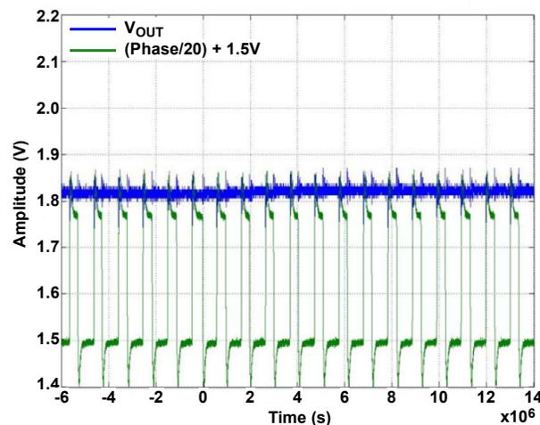
Figure 36. Set Response with 5.5V Input,  $\Delta V_{OUT} < 1\%$
