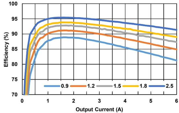
Figure 7. 3.3V  $V_{IN}$  Efficiency for Multiple  $V_{OUT}$  Levels
