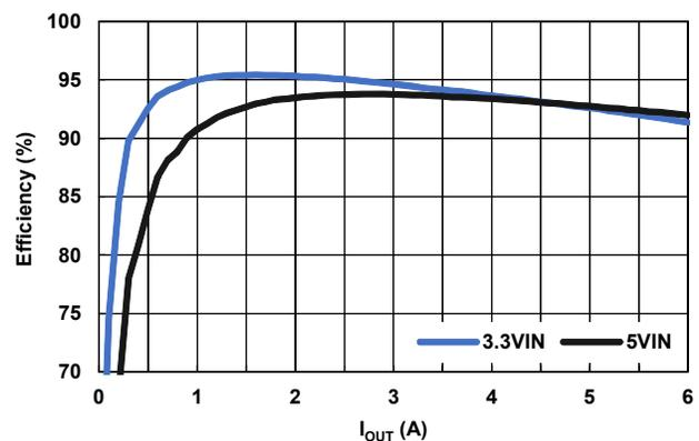
Figure 2. Efficiency vs V<sub>IN</sub> for 2.5V Output, T<sub>C</sub> = +25°C
