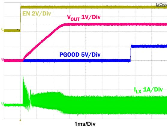
Figure 15. Start-Up to 2.5V  $V_{OUT}$  Waveforms  $I_O = 0\text{A}$
