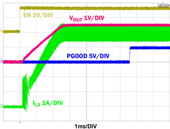
Figure 16. Start-Up to 2.5V  $V_{OUT}$  Waveforms  $I_O = 5\text{A}$
