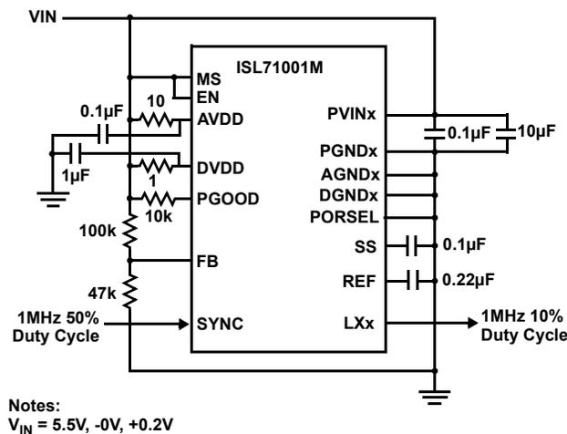
Figure 30. Irradiation Bias Configuration for the IS71001M
