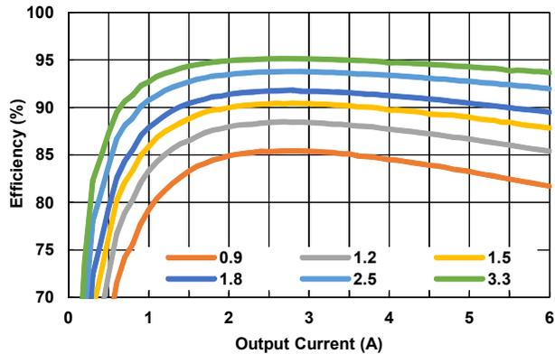
Figure 6. 5V  $V_{IN}$  Efficiency for Multiple  $V_{OUT}$  Levels
