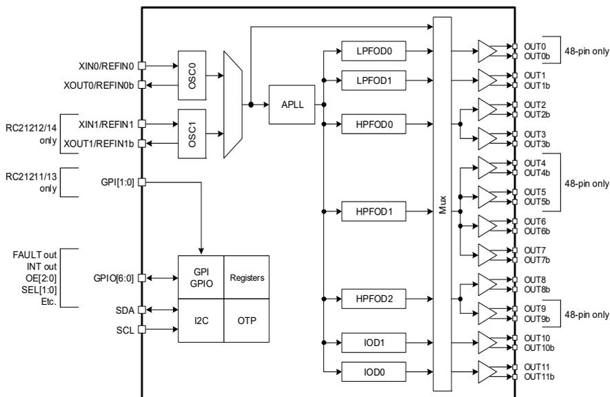
Figure 1. RC2121xA Block Diagram
