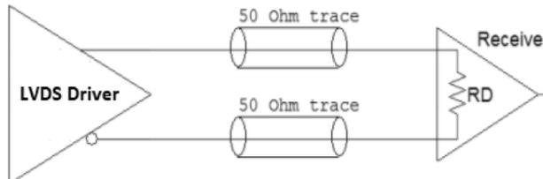
Figure 11. Standard LVDS Termination
