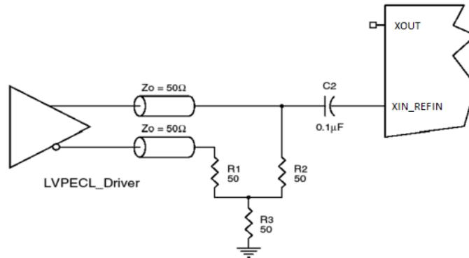
Figure 9. LVPECL Driver to XTAL Input Interface
