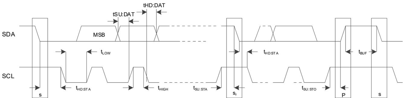
Figure 4. I<sup>2</sup>C Slave Timing Diagram
