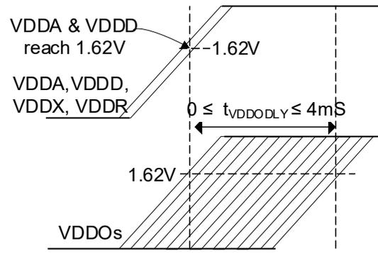
Figure 13. Power Supply Sequencing without PWRGD/PWRDN# or PWRGD/RESTART#
