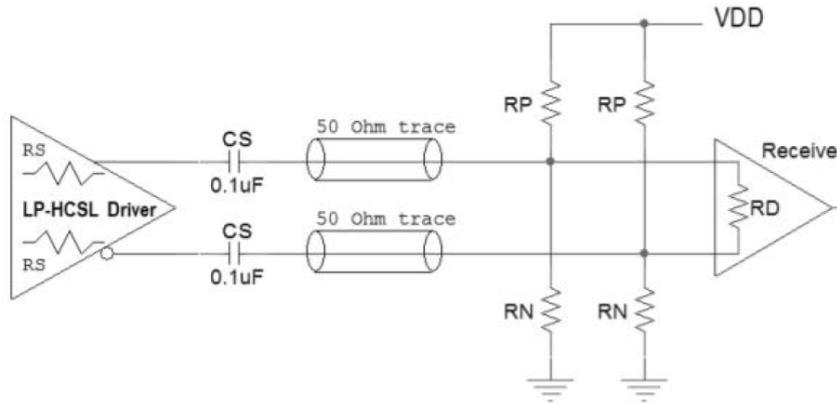
Figure 12. AC-Coupling Termination
