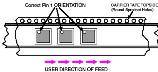
Figure 15. Pin 1 Orientation in Tape and Reel Packaging
