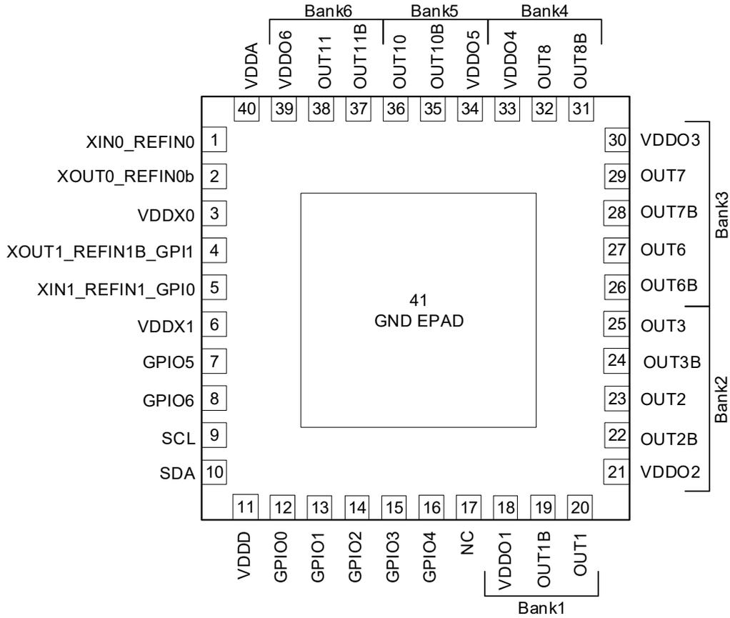
Figure 3. 40-QFN (5 × 5) Pin Assignments – Top View
