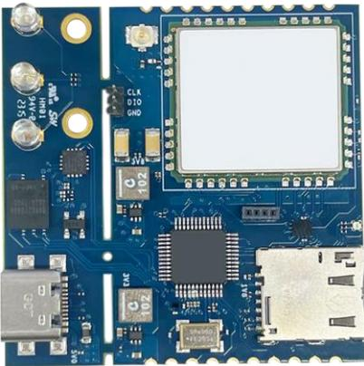
monoZ is a strategic partner for 1NCE, a global MVNO offering managed connectivity services for low-bandwidth IoT applications. monoZ:Jet is a 1NCE compatible compact low-power solderable System-on-Module (SOM) that enables secure IoT connectivity to user system. monoZ:Jet acts as data pump that push the incoming data from host system to the monoZ:Link IoT cloud platform. It is a ready to use device with preloaded application firmware and can be integrated in different user systems.
