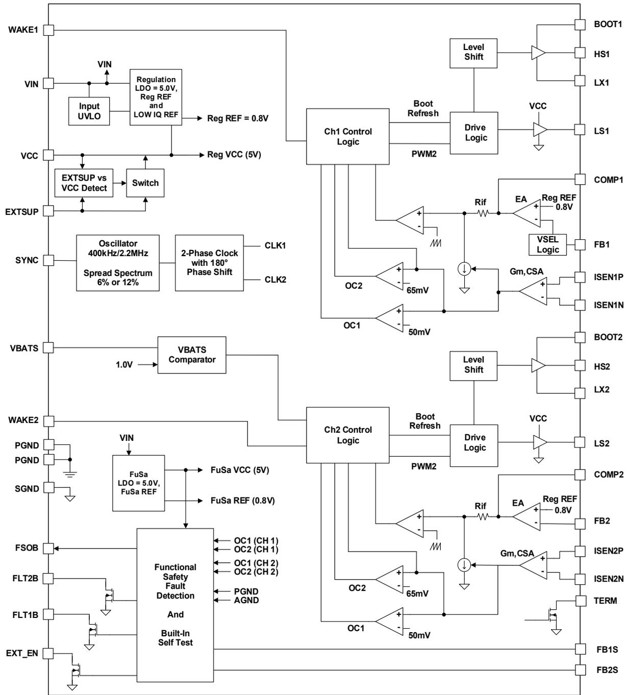
Figure 2. Block Diagram
